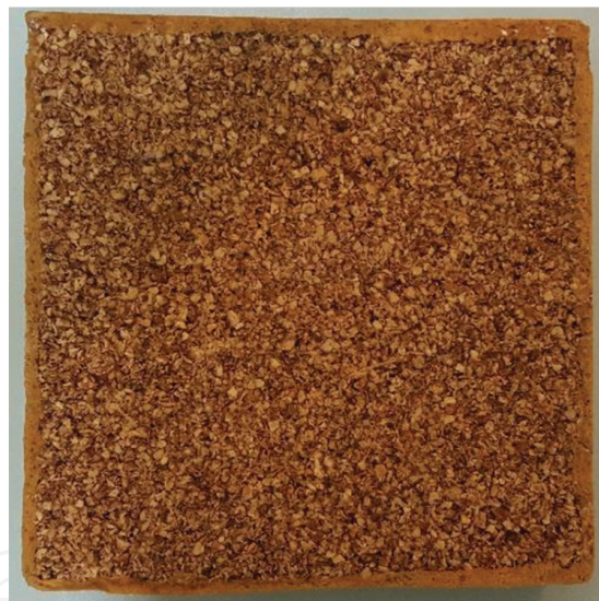
Figure 11. A sample of a 3-cm-thick corncob particleboard.
