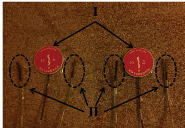
Figure 8. Granulated corncob sample under thermal insulation performance test (I: heat flux sensors and II: superficial temperature sensors).
