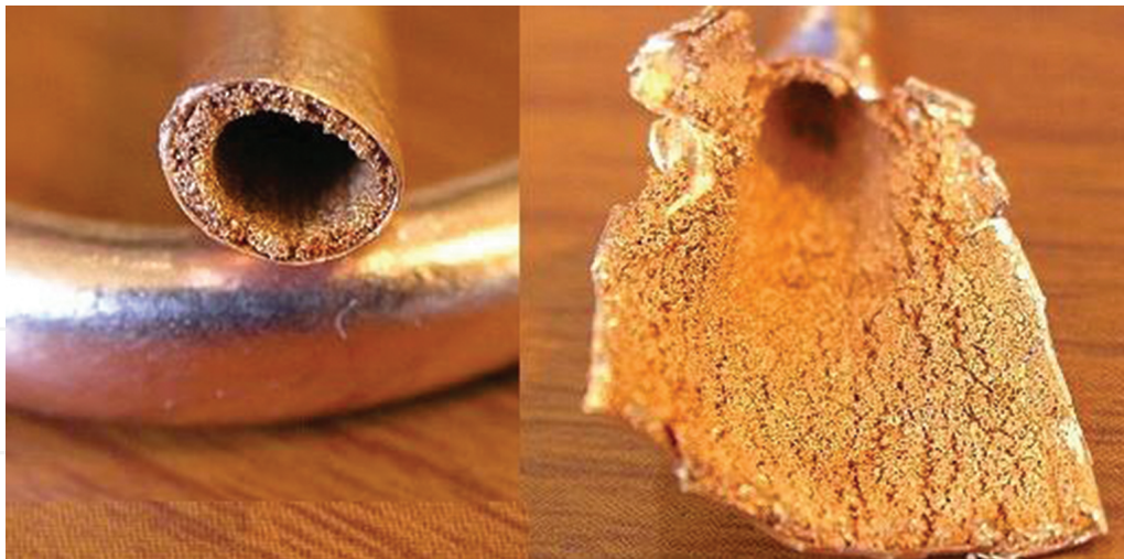
Figure 2. Metal sintered powder wick [15].
