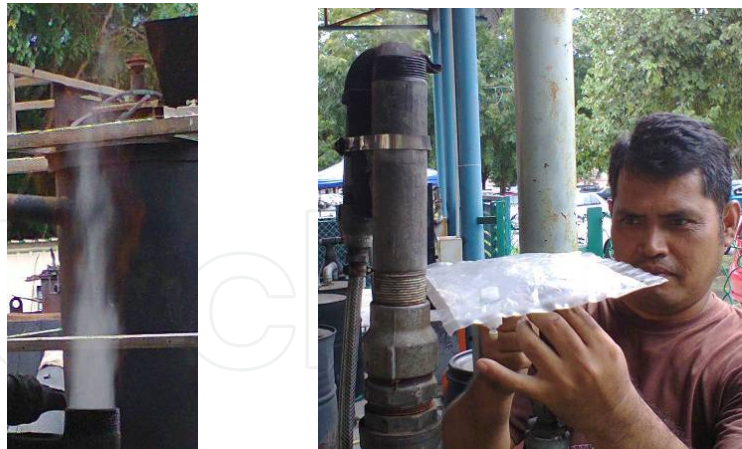
Figure 9. Flare (left) and gas sampling for analysis (right).
