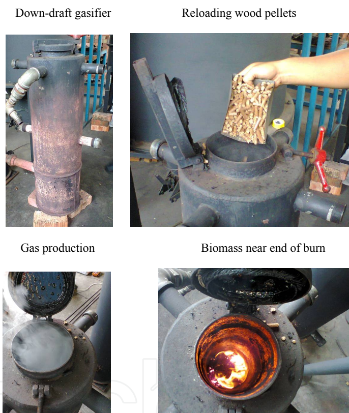
Figure 8. USM's 5 kW down-draft wood pellet gasifier.
