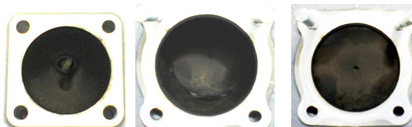
Figure 15. Cylinder head (left) bore (center) and piston crown (right) indicating significant tar or soot buildup, especially at the colder locations.
