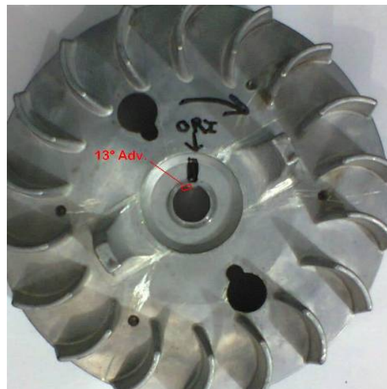
Figure 4. Flywheel with mark indicating new keyway providing spark advance.
