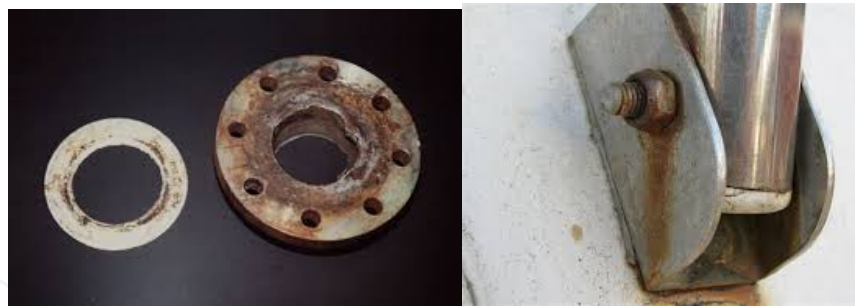
Figure 4. (a) Crevice Corrosion on a Steel Flange [17] and (b) Typical View of Crevice Corrosion.
