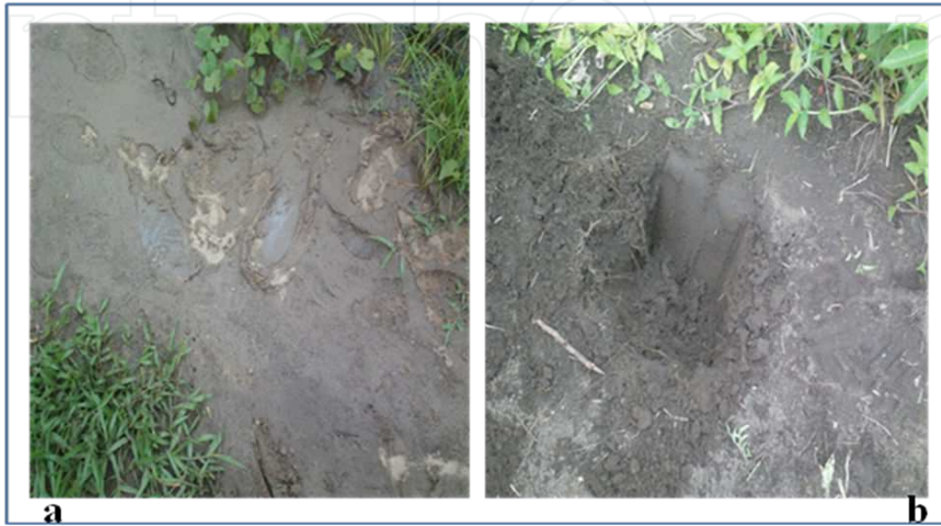
Figure 14. Reduced water infiltration in Subsite B (RMS) relative to the agricultural farm soil (Subsite C: AGS)
