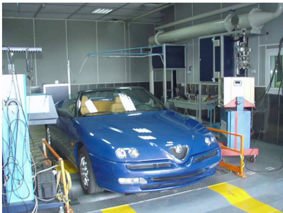
Figure 4. Chassis dynamometer SCHENCK 500GS/60 in BOSMAL Automotive Research & Development Institute
