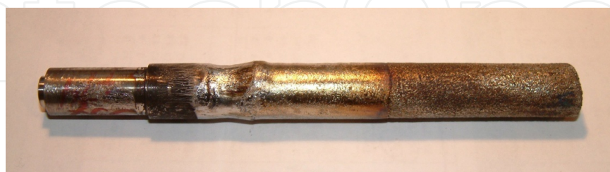
Figure 9. Erosion traces of the IPD accelerator internal electrode.
