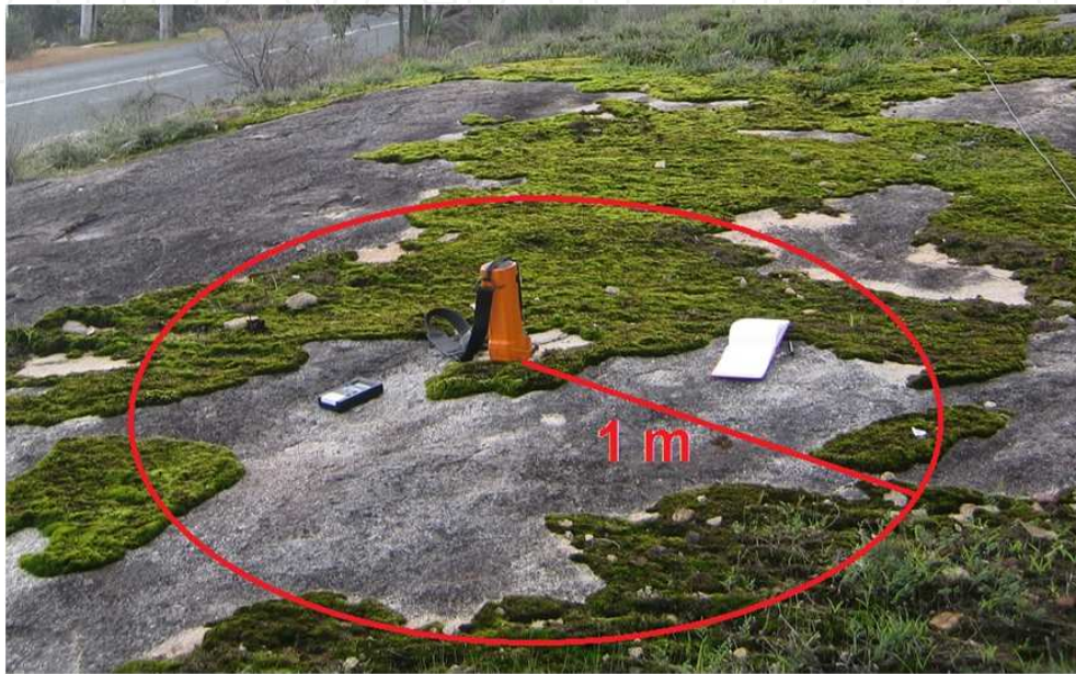
Figure 4. A diagram showing the RS-125 sampling zone, which is essentially a 1-m-radius hemisphere below the earth's surface.
