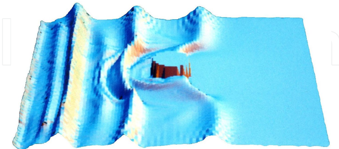
Figure 2. Perspective of the free surface obtained by simulation around the Bugio lighthouse, situated in the Tagus estuary, Portugal, in a transient condition.
