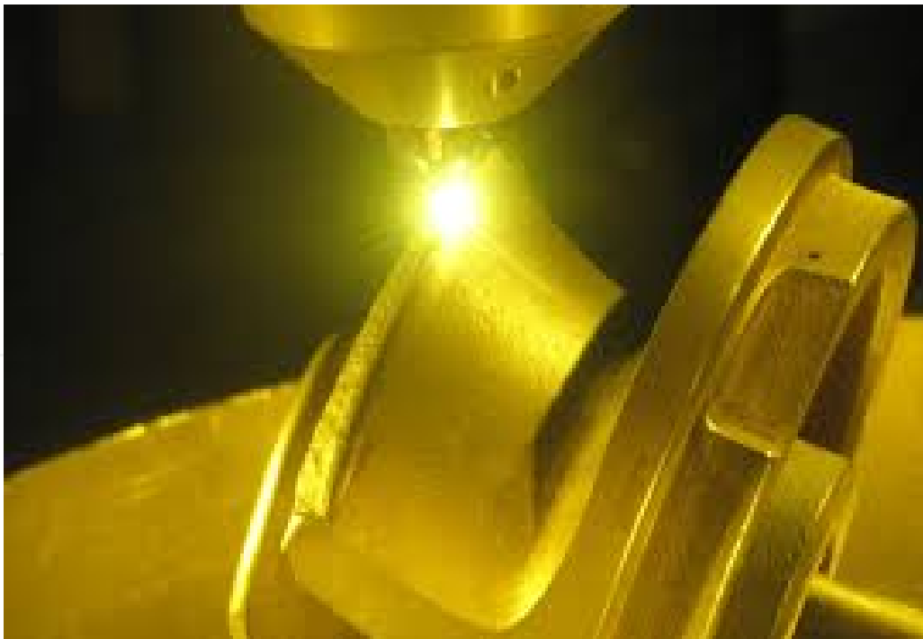
Figure 8. Fabrication of impeller pump using LENS™ [40].
