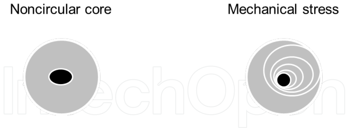
Figure 2. Fibre cross-sections with cylindrical symmetry broken by manufacturing process that leads to fibre birefringence.
