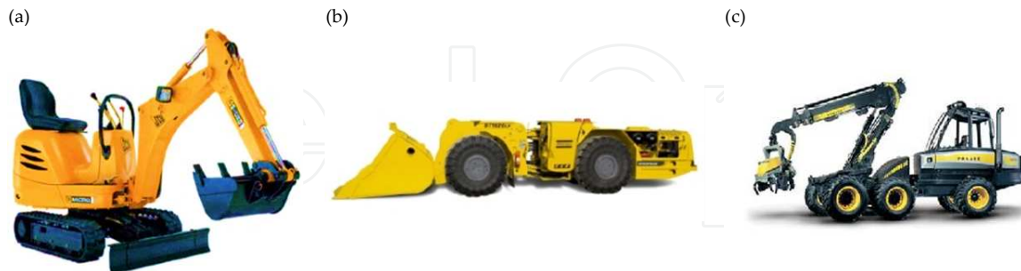
Figure 1. Examples of non-road mobile machinery: (a) excavator; (b) mine loader and (c) forest harvester.
