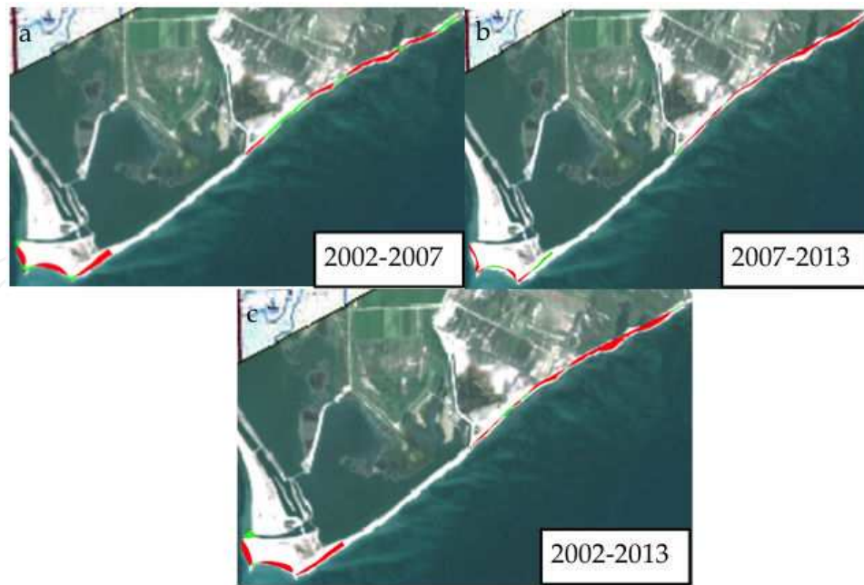
Figure 6. Erosion (red color) /Accretion (green color) balance at Akroneri Cape region
