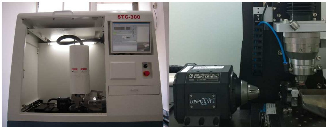
Figure 5. Integrated laser module with a magnified view of the linear X-Y motor stage and laser source in the right window.
