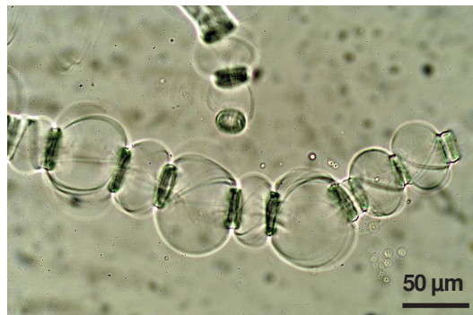
Figure 2. Wood fiber swollen by “ballooning” in NMMO – 20 % w/w water at 90 °C (magnification of 200 times). (Pictures were taken by NLM at CEMEF - MINES ParisTech)
