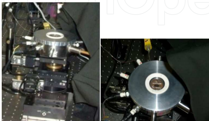
Figure 9. Experimental sample cell used to probe SHG signal as a function of temperature. It allows measurements either in air or vacuum, and for alignment purposes it is positioned on a mirror mount attached to the rotation/translation stage.
