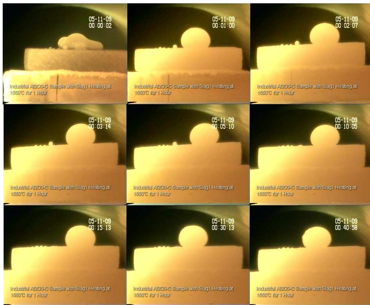
Figure 18. Industrial flat oxidized \text{Al}_2\text{O}_3\text{-C} samples with slag 1 heating at 1550^\circ\text{C} for 1 hour
