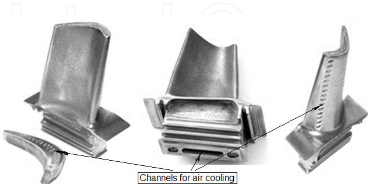
Figure 1. Air-cooled and thermal barrier-coated high-temperature turbine blade for turbojet engine Al31-F.
