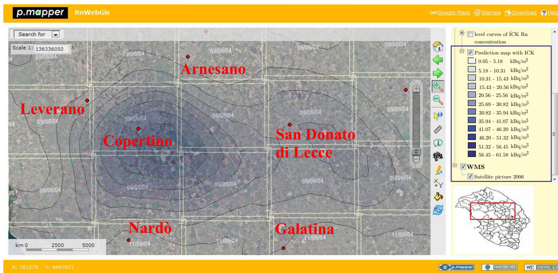
Figure 13. Orthophoto of Lecce district, obtained by the WMS and integrated with the “Rn sites”, “level curves of ICK” and “Prediction map of ICK” layers.
