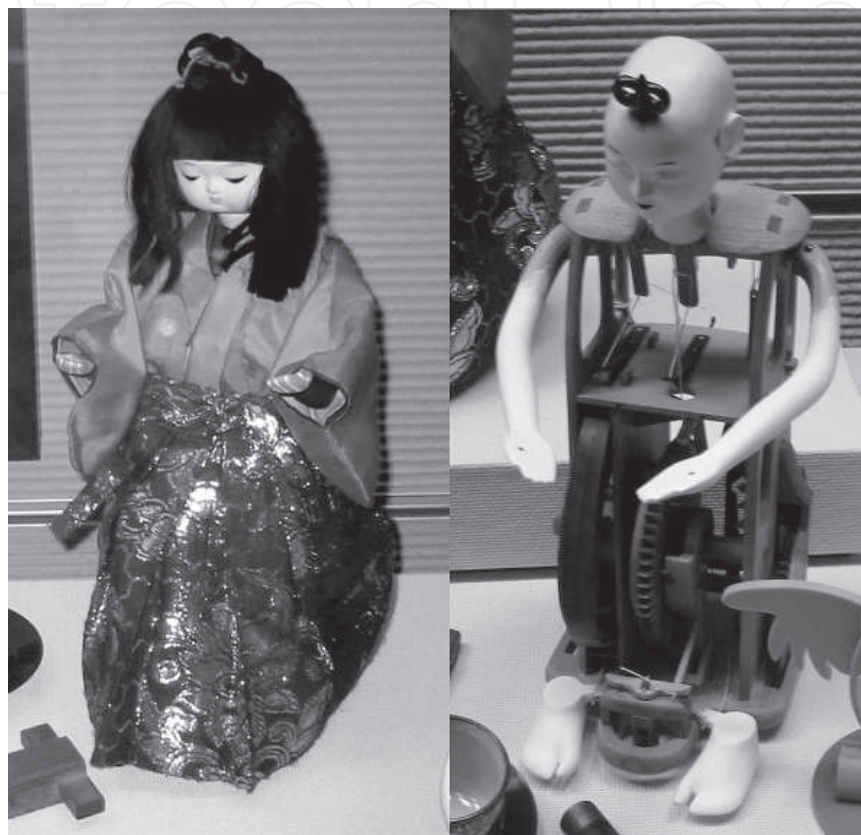
Figure 1. Karakuri ningyou (Japanese mechanized doll). This is a tea serving mechanized robot. The karakuri ningyou serves a cup of tea, and its sequence is roughly as follows: 1) When a cup of tea is placed on the hands, they start to move toward a guest by moving its feet like walking. 2) It moves, setting distance, and bows its head. 3) When a cup of tea is taken from the hands, it stops and waits for a next action. 4) It turns around and returns to the starting position (host's place) when an empty cup is placed on the hands. It works by springs. Only the examination of each mechanical gear would not help to understand the entire behavior of the doll. Picture is taken from Wikimedia Commons [3] and converted to gray scale
