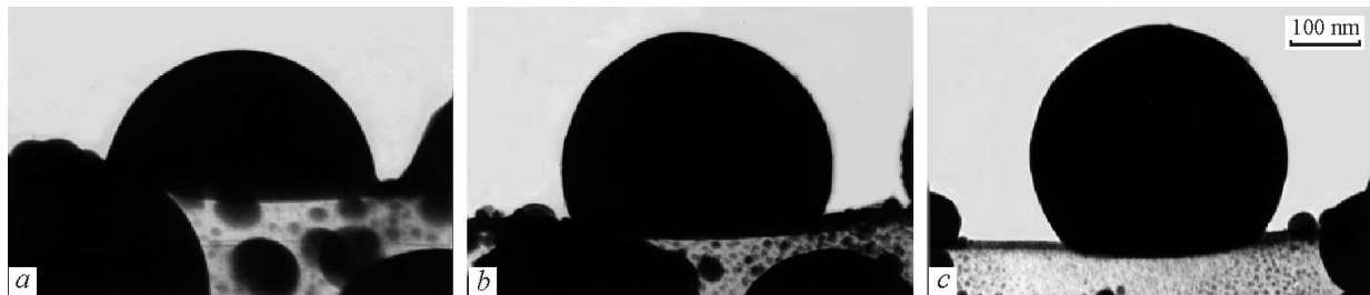
Figure 16. Micrographs of crystallized tin droplets condensed in a vacuum of 2 \cdot 10^{-8} mm Hg on carbon substrates at temperatures 350 K (a), 410 K (b), and 500 K (c) [42, 43, 77]
