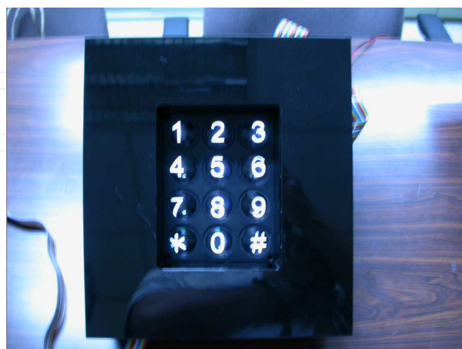
Figure 24. Top view of the floating image system.
