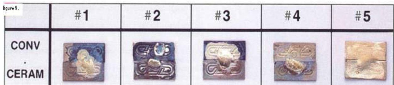
Figure 9. Illustration of galvanic corrosion observed in the 5 samples (1-5)
