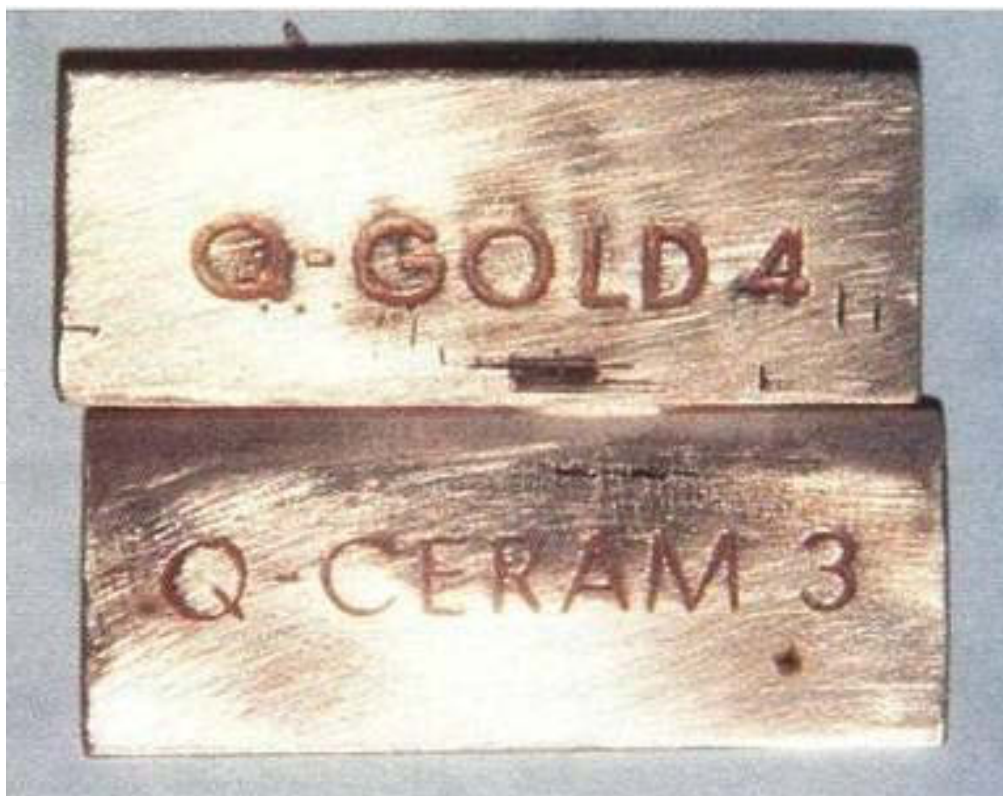
Figure 8. The corrosion test samples are two plates of noble alloy connected by soldering
