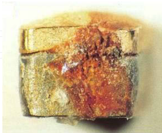
Figure 1. Bimetallic wrist bracelet made of bimetallic rings gold/steel after corrosion in saline solution
