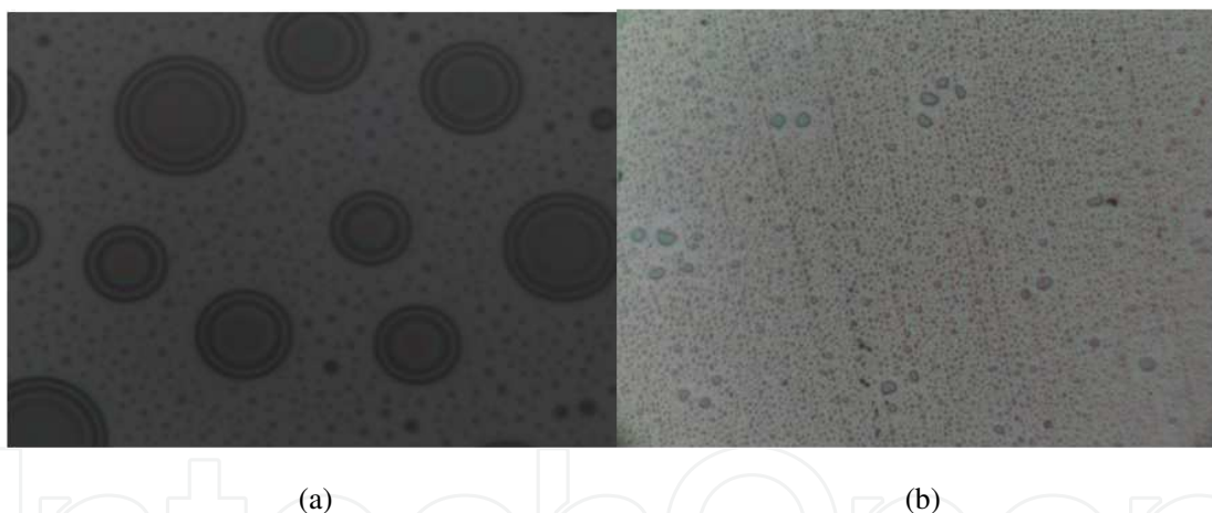
Figure 18. Optical microscopy images of the substrates after the deposition of the droplets: a) glycerol on mica; b) glycerol on stainless steel. Field of view \sim 80 \mu\text{m} \times 64 \mu\text{m}
