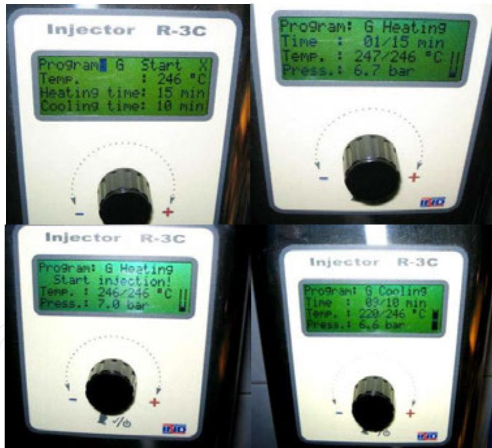
Figure 12. Schedule of “G” program of injecting the thermoplastic material (a) Start (b) Heating (c) Injecting (d) Cooling
