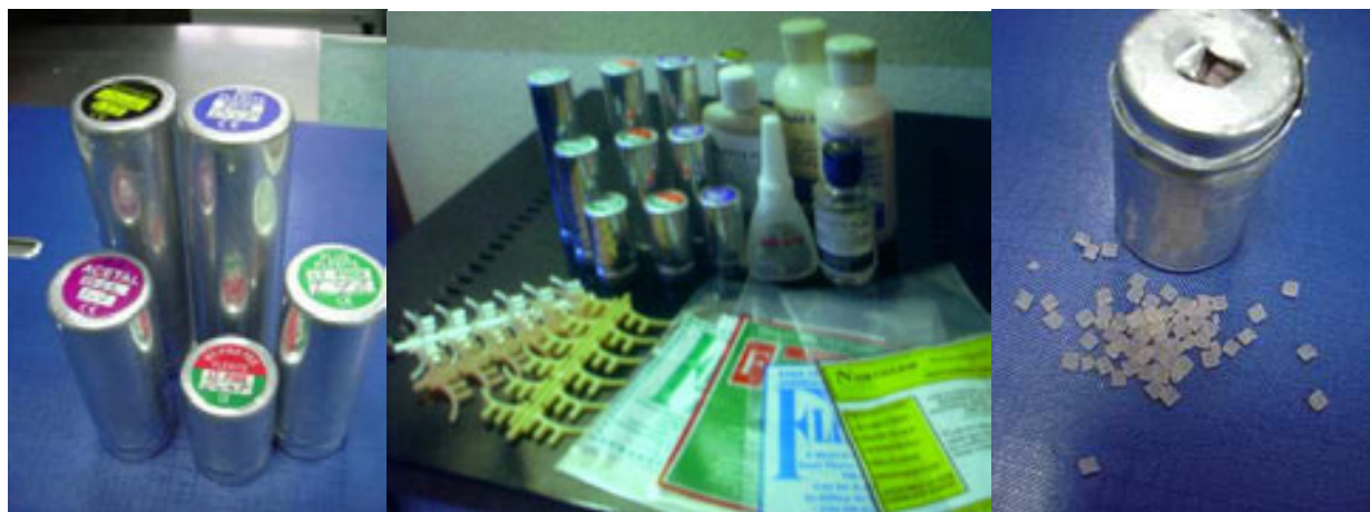
Figure 3. (a, b) Cartridges of different thermoplastic resins (c) The granular aspect of the material
