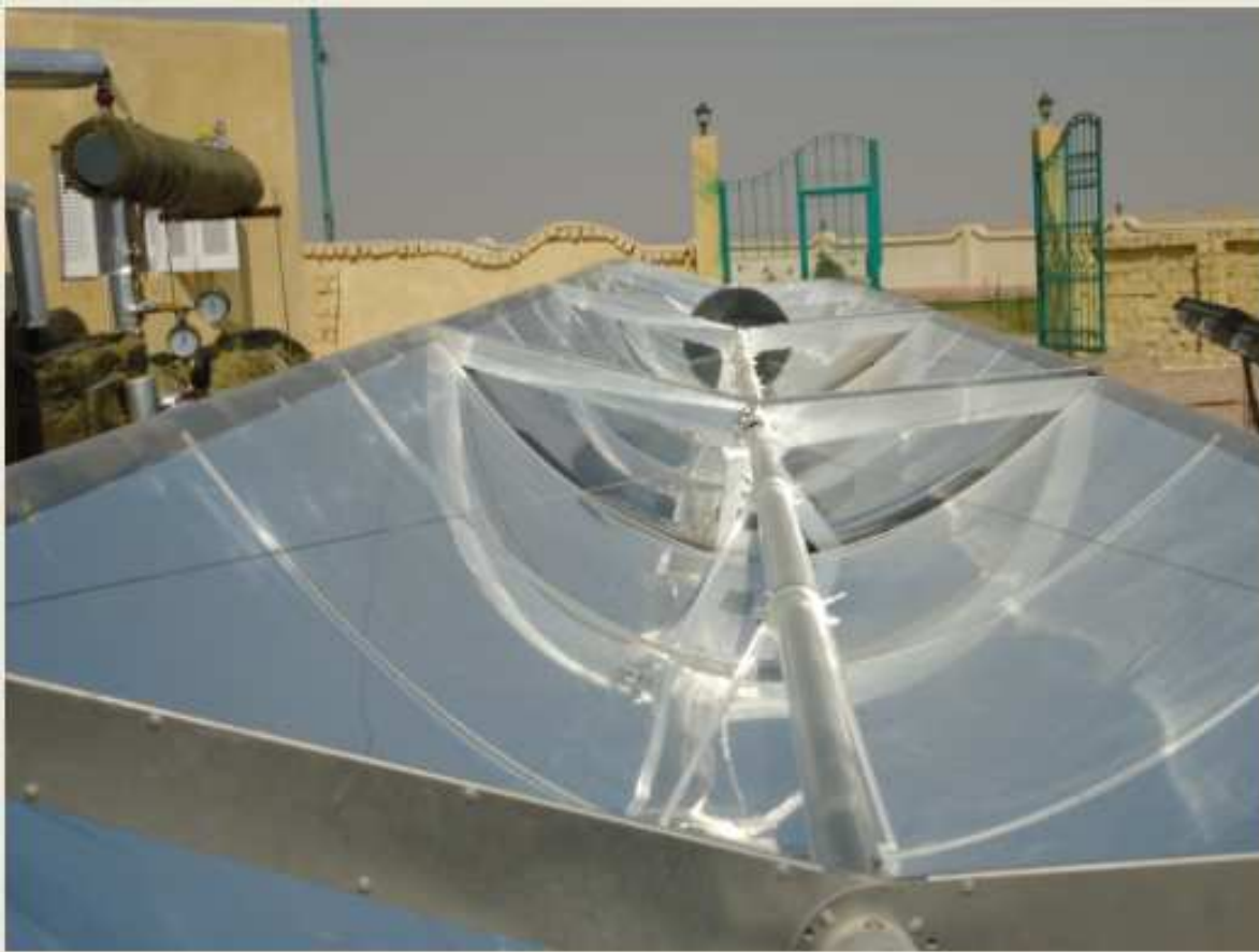
Figure 22. Four modules of the concentrated solar collector in series [13]
