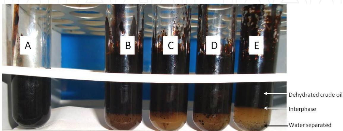
Figure 8. Photographs showing separated water (WS) from the initial O/W emulsion containing GlyC 12 (1000 ppm) at 50 W, 60°C. Initial O/W emulsion before MW irradiation (A), emulsion after MW irradiation during 2 (B), 4 (C), 8 (D), 10 minutes (E).
