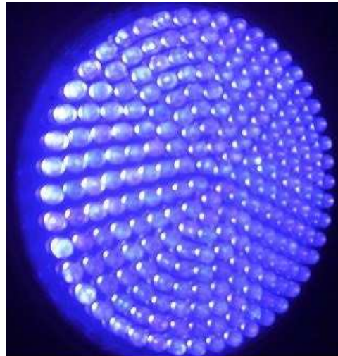
Figure 2. Arrangement of high brightness LEDs that emit blue light.
