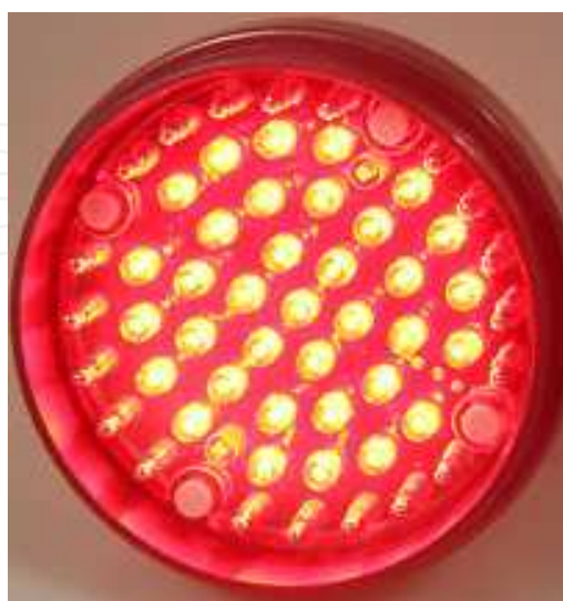
Figure 1. Arrangement of high brightness LEDs that emit red light.
