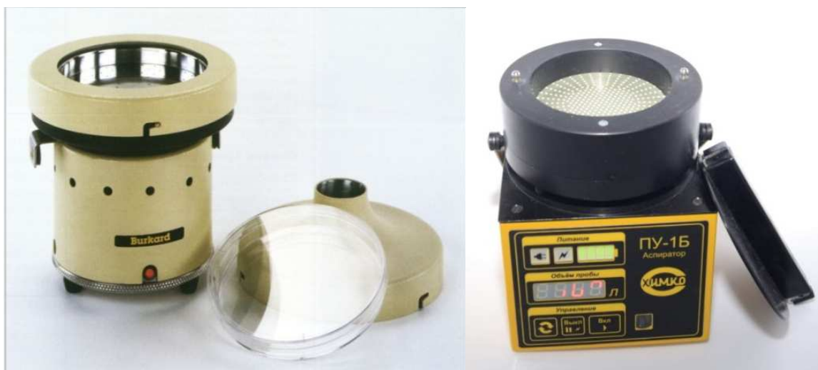
Figure 4. Burkard SporeWatch sampler and sampler (St. Petersburg) PU-1B The determination of the spores concentration (colony forming units-CFU) in the atmospheric air of the premises, parks and industrial areas is also very informative for collecting the patient's medical history and selection of diagnostic tests in vivo and in vitro.
