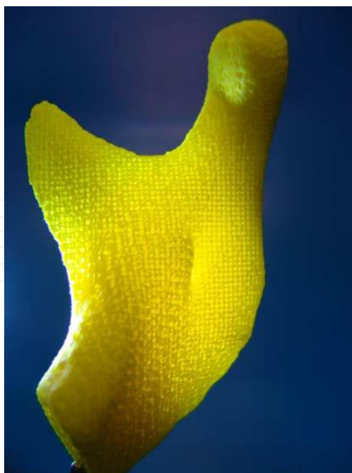
Figure 1. Printed mandibular condyle by Fused Deposition Modeling (FDM) process. Image provided by Centro de Tecnologia de Informação (CTI) – Renato Archer (Campinas, Brazil).
