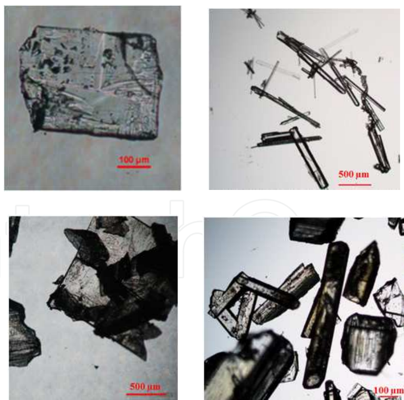
Figure 14. Optical micrograph of phenacetin recrystallised from (top left) dichloromethane, (top right) ethanol, (bottom left) water and (bottom right) acetonitrile.
