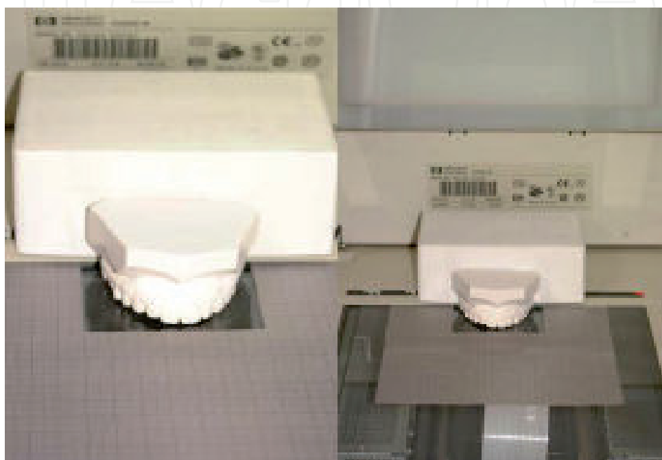
Figure 1. Guidance and scanning study models in the scanner in the Digital Method.
