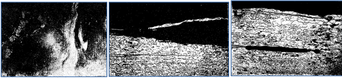
Figure 20. Swelling of a hot-rolled tungsten sheet from the 'low' density ingot, annealing for 2 h in hydrogen at 1500°C: (a) ingot surface ( \times 2 ); (b) transverse section, subsurface discontinuities is seen ( \times 80 ); (c) pore with hydrogen, looks like elongated "bubble" after annealing, splitting cracks are seen ( \times 100 ).
