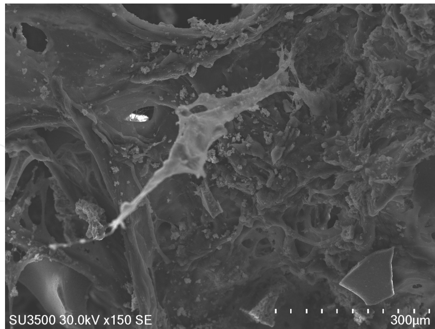
Figure 21. SEM Evaluation of MSCs ( \times 50 ). SEM analysis shows lodging of the cells within the pores of the scaffold.
