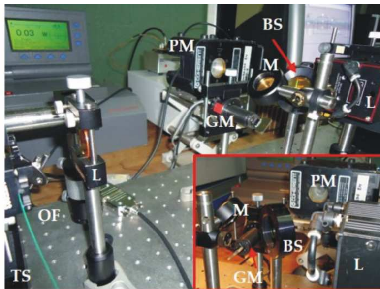
Figure 8. Picture of the setup implemented. The inset shows a detail view of the laser output area. BS – beam splitter; CL – cylindrical lens; GM – galvanometric mirror; L – laser; M – mirror; OF – optical fiber; PM – power meter; TS – translation stage.
