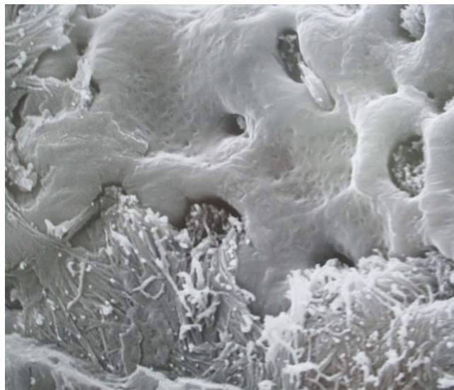
Figure 3. SEM view of TiUnite surface when osteoblasts have filled pores on the implant surface.
