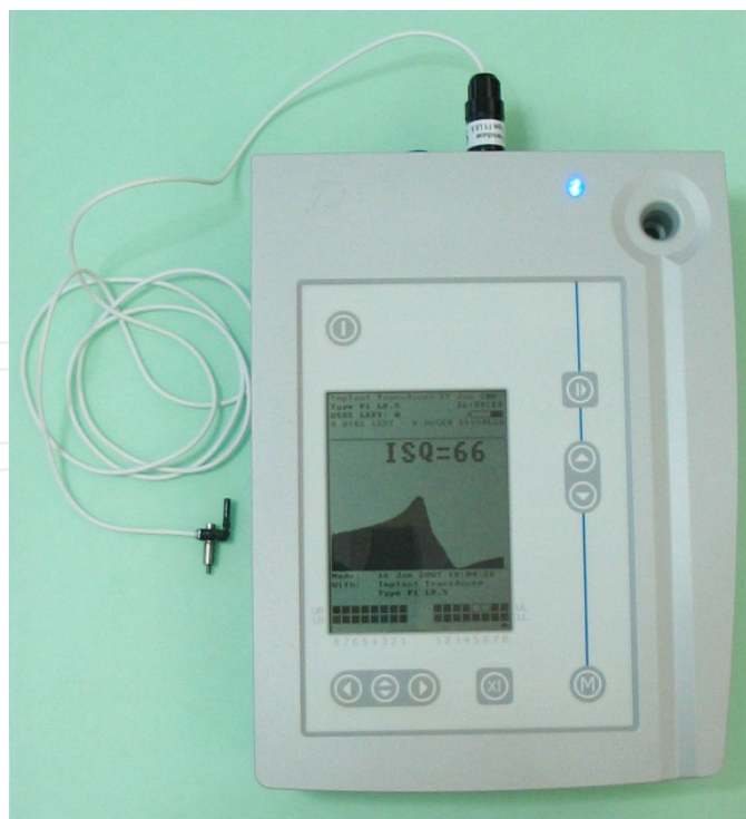
Figure 14. Osstell instrument used to determine implant stability.
