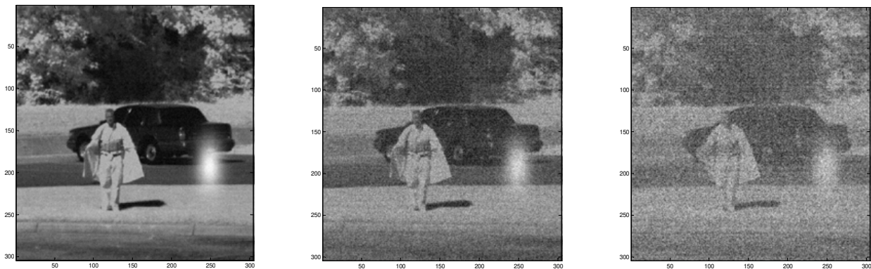
Figure 5. Atmospheric effects on clear night sky. NIR images at distances of 1, 10, and 15 km (left to right) for 5 km visibility conditions.
