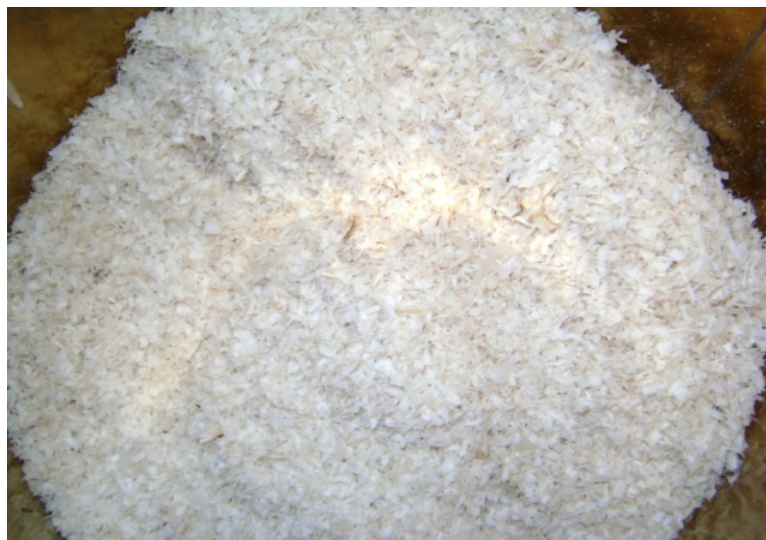
Figure 11. Charred organic impurities on pre-heating the shredded scrap
