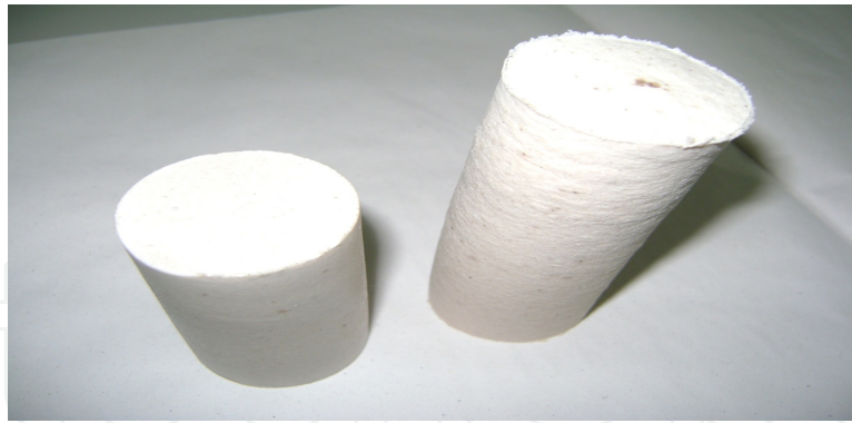
Figure 19. Reprocessed PTFE filled (40%) PTFE pellet before (left) and after (right) sintering at atmospheric pressure. The surface became rough on sintering due to agglomeration of reprocessed particles and their migration to surface of the pellet. Reprocessed PTFE is amenable to sintering only under pressure or under ram extrusion.
