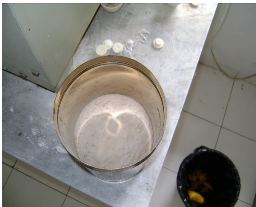
Figure 15. Ground scrap powder after pre-sintering
