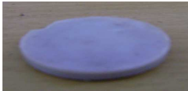
Figure 24. Repro filled PTFE Discs when sintered inside the die and plunger under C-clamp show discoloration which runs through its volume although good surface smoothness is seen and cracks disappeared totally. This was attributed to carbon production on reaction of volatiles with the die material. Even 100% virgin PTFE pellet show slight discoloration but only on its surface (both sides) when sintered under C clamp
