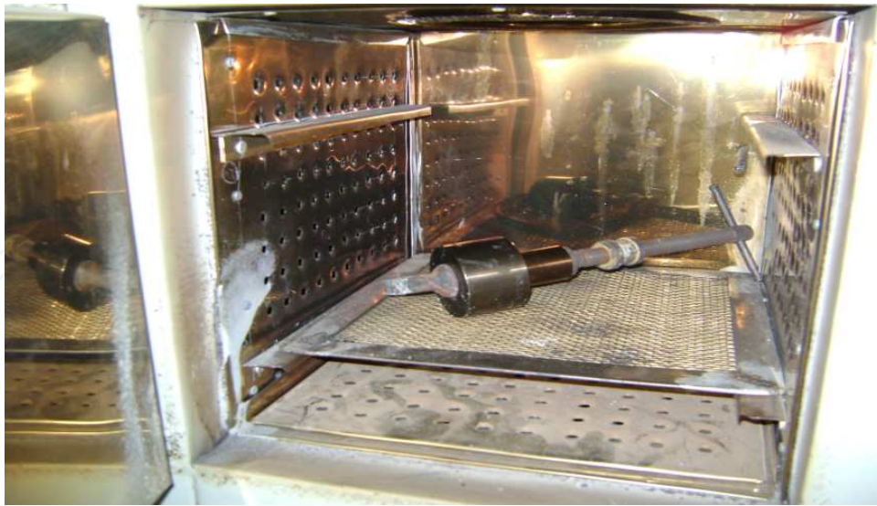
Figure 23. Die under C-clamp kept inside the air over for sintering near 400°C
