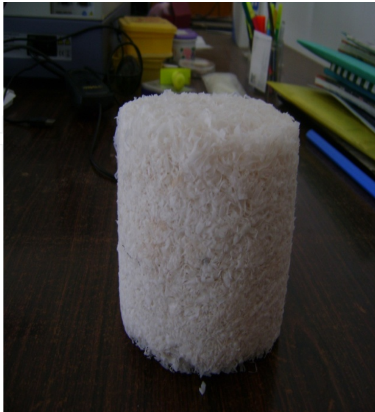
Figure 13. Shredded PTFE scrap after pre-heating treatment
