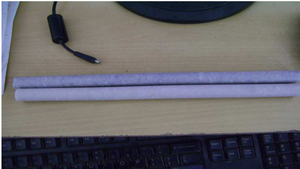
Figure 28. A 40% repro + 60% virgin PTFE mixture was ram extruded into long rods of diameter 17 mm with the help of a local industry in India. The rods came out fine from the points of polish and strength but was dark in color with patches all through the length and volume due to carbon deposition.
