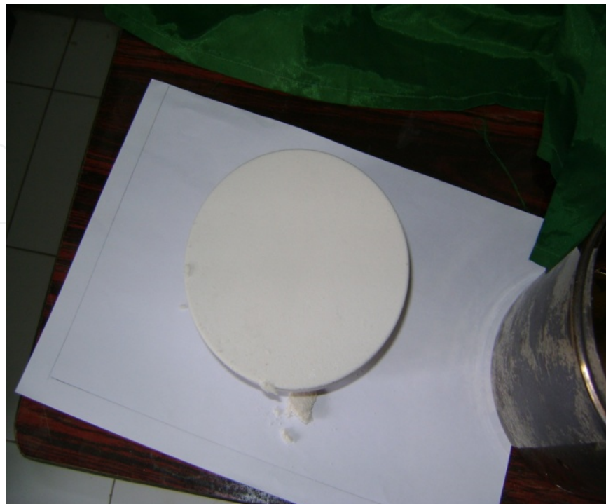
Figure 14. Pre-sintered scrap powder
