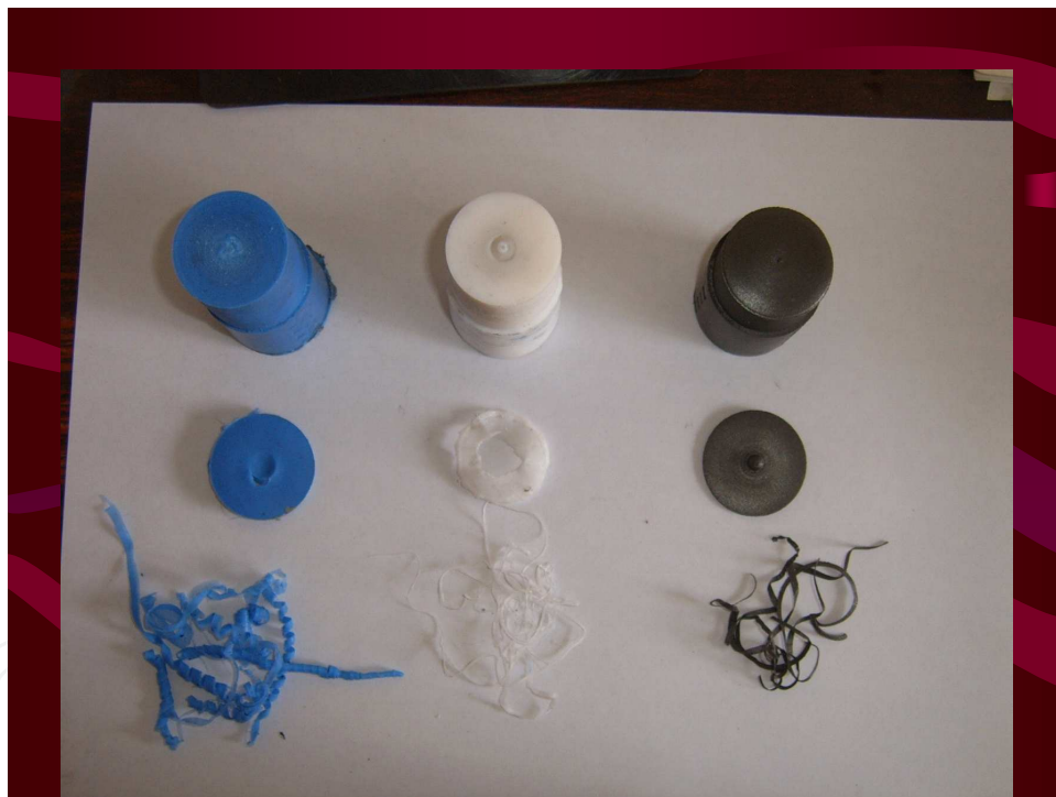
Figure 5. Sintered rods made from blue pigmented PTFE, glass mixed PTFE and carbon mixed PTFE
