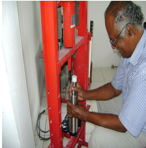
Figure 17. Mixture being cold pressed into pellet.
