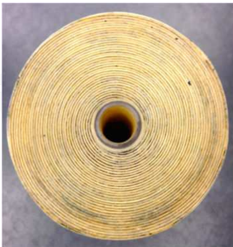
Figure 6. Used RO membrane from a home dialysis WRO machine
