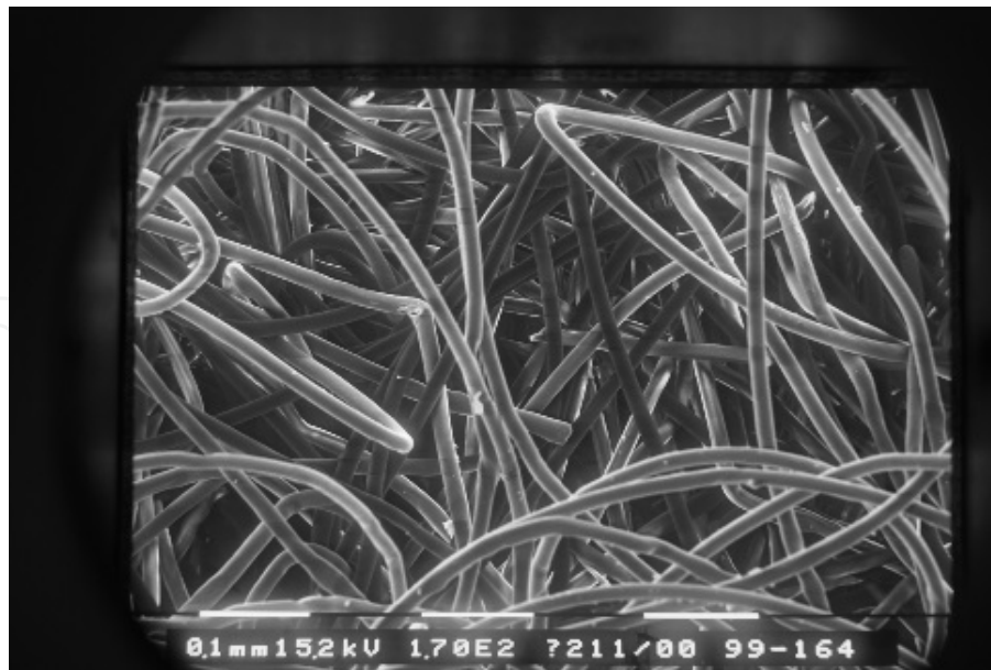
Figure 4. Biodegradable PGA felt, with open “spaghetti”-like structure. 170X
