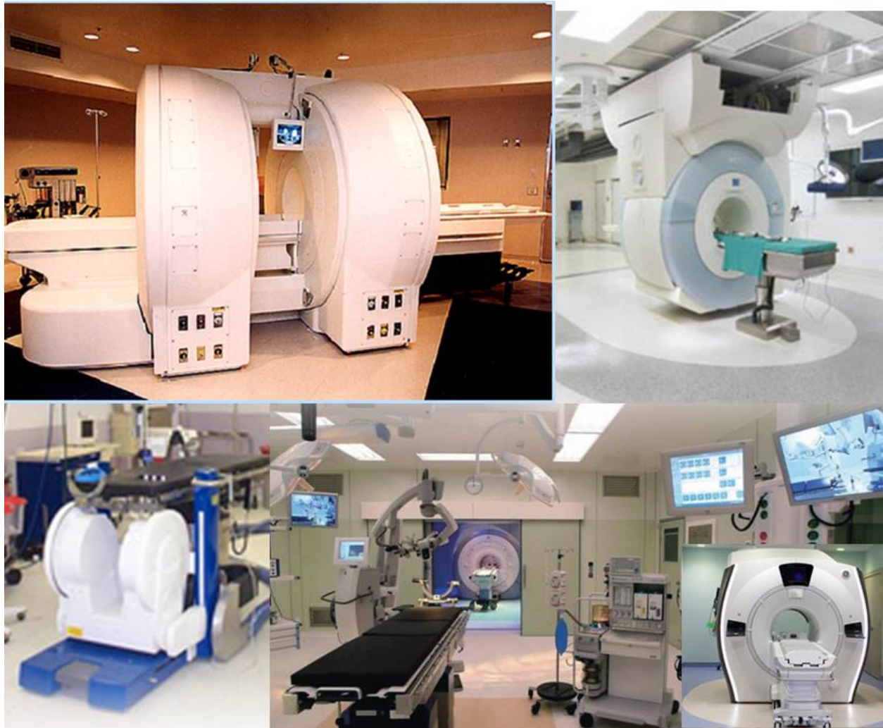
Figure 5. Various Intraoperative MRI concepts (clockwise from top left: GE Signa SP double doughnut, IMRIS mobile ceiling mounted system (scanner moves to patient), GE hybrid OR concept (inset shows close up of scanner; patient moves to scanner), Odin table mounted system).
