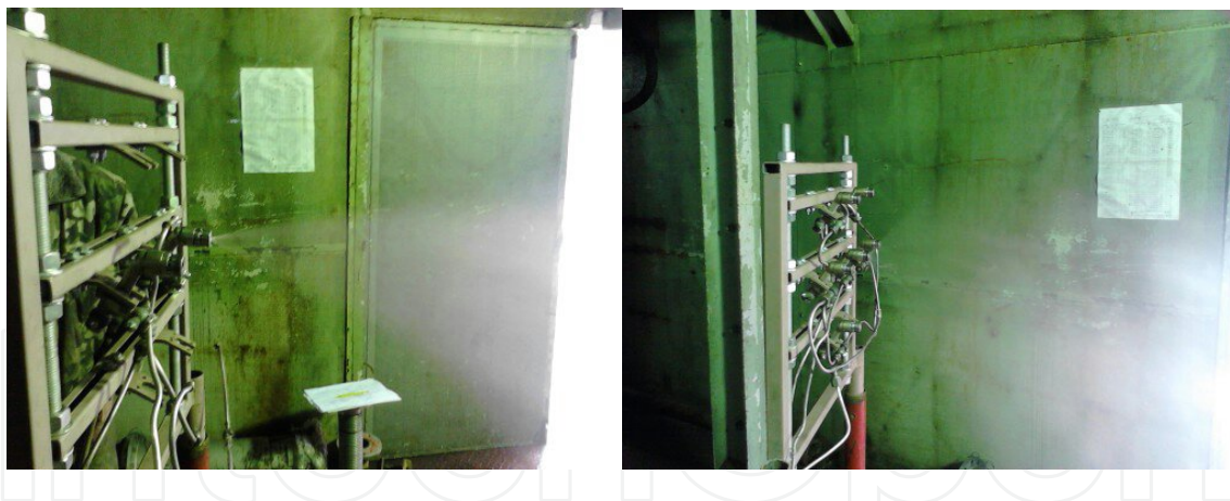
Figure 17. Water spraying tests, using a liquid fuel atomizer from TV2-117A gas turbine
