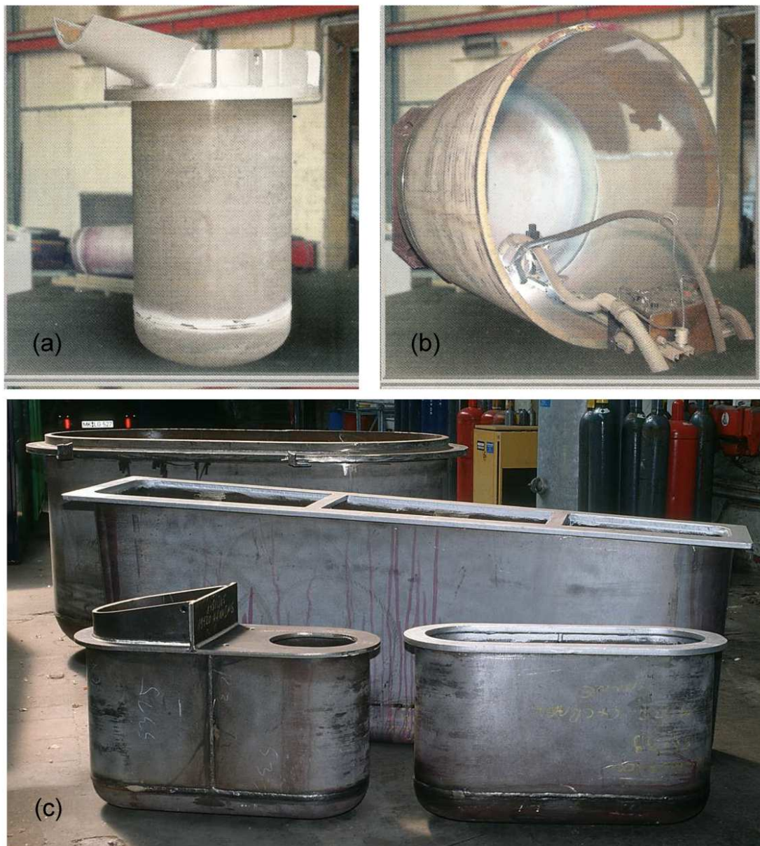
Figure 9. Commercial processes requiring equipment resistant to liquid magnesium: (a, b, c) crucibles for magnesium melting [83];
