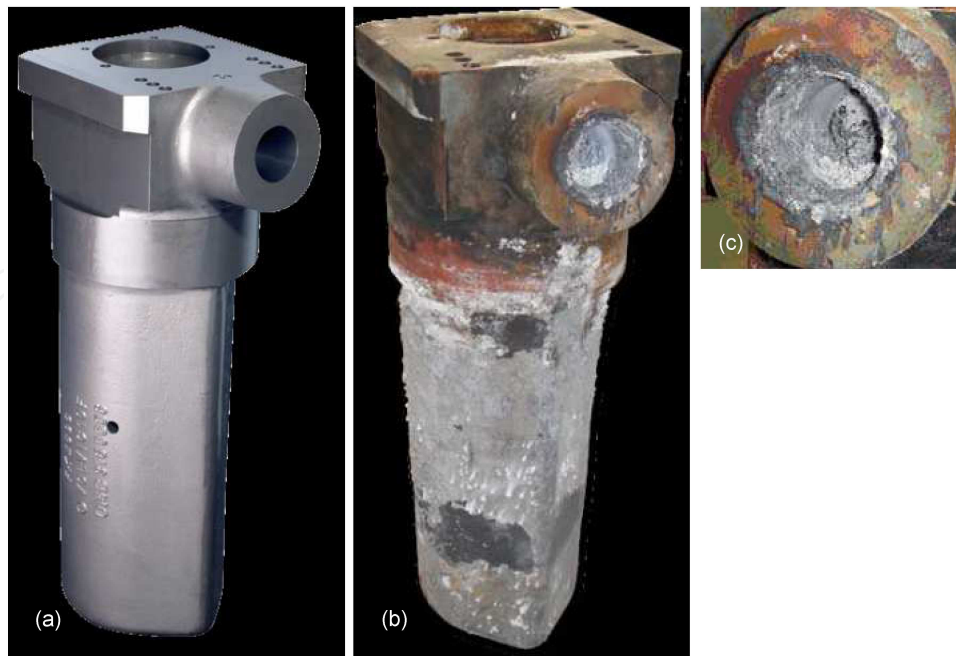
Figure 16. Goosenecks of hot chamber die casting machine: (a) part before exposure to liquid magnesium; (b, c) gooseneck after service with extensive corrosive attack [85].
