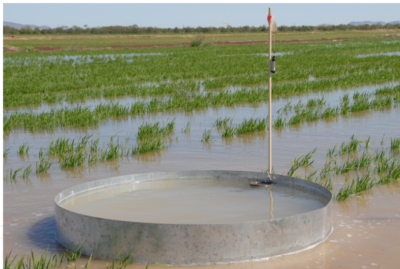
Figure 5. Class A Evaporation Pan with a stilling well located near one edge (also shown is a Baro-Diver to measure variations in atmospheric pressure).
