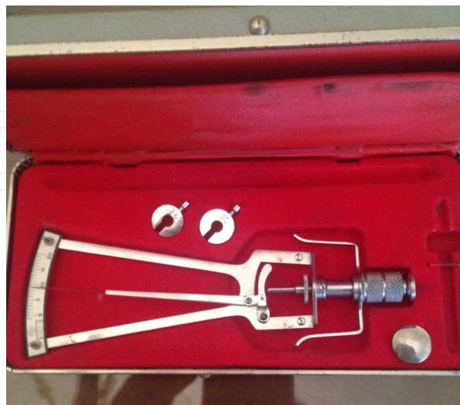
Figure 1. Schiötz tonometer of known weight
