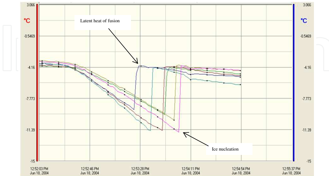
Figure 12. Temperature profile using nucleation manifold. Thermocouples were placed in the corner wells and middle wells of a 96 well plate. Temperatures were recorded every few seconds.
