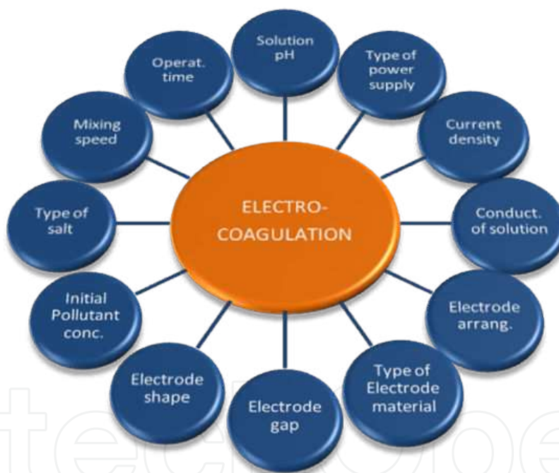
Figure 3. Schematic display of the various operating parameters influencing the EC process performance.
