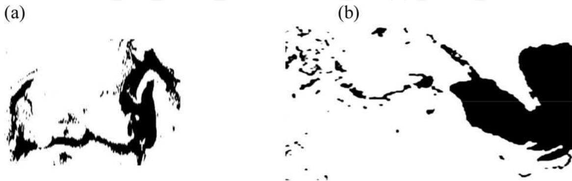
Figure 11. Oil spill automatic detection by Genetic Algorithm (GA) using (a) RADARSAT-2 SAR and (b) ENVISAT ASAR in Gulf of Mexico
