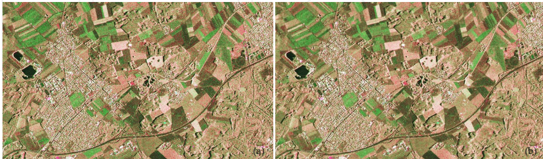
(a) color composition of the unfiltered HH (red) and VV (green and blue) amplitudes. (b) color composition of the speckle filtered HH and VV amplitudes obtained using the Gaussian-DE MAP filter for series of multilook detected SAR images (cf. § 5.5.1).
