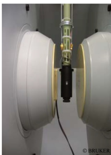
Figure 5. Electromagnet and the resonance cavity of CW-EPR spectrometer produced by Bruker BioSpin GmbH.
