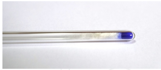
Figure 9. Ultramarine in the glass tube to EPR measurements.
